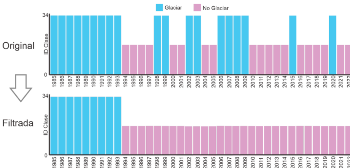
Figure 12 - Effect of applying the temporary permanence filter
